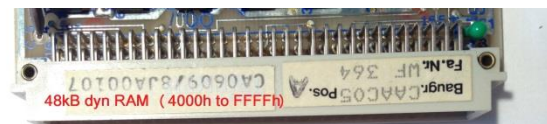
ADAPTER: Addresses access 0000h-BFFFh shift range / hide selection 0000h-3FFFh (off/on) software switching
